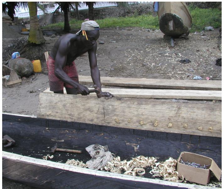
**ANATOMY OF A FISH BOAT.** The planks are three inches thick and 10 inches wide. Tropical wood is so excellent as it doesn't split, it's easy to drive nails into, and it lasts and lasts. The boat of course weighs a couple thousand pounds.
